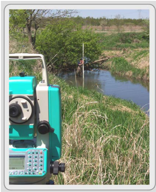
Figure 2.2: Total station, a surveying instrument, measures distance, direction, and location. Image comes from Illinois State University, Geography Dept.
