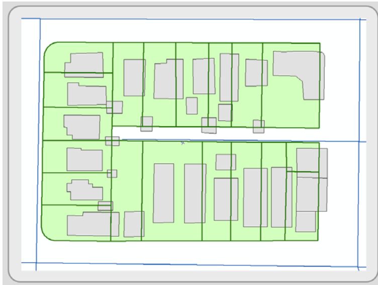
Figure 2 6: Due to differences in the projection parameters of the parcel layer, it is not lining up properly with the street centerline and buildings layers.
