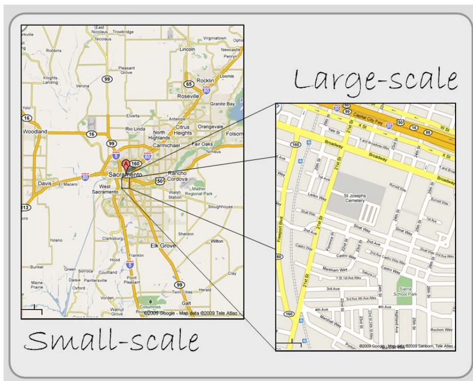
Figure 2.3: Map scale. Small-scale maps depict larger territories, but large-scale maps present more detail.
